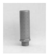
Product description The blow-off silencer consists of a tube with a closed end in which a large number of small holes have been made, the number, the diameter and the pattern of the holes are determined by the required silencing
